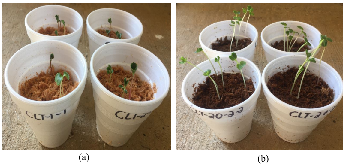
Figure 4.7 Overall visual germination results of CLT (a) and CLT 20 (b) with radish seeds at day 150
